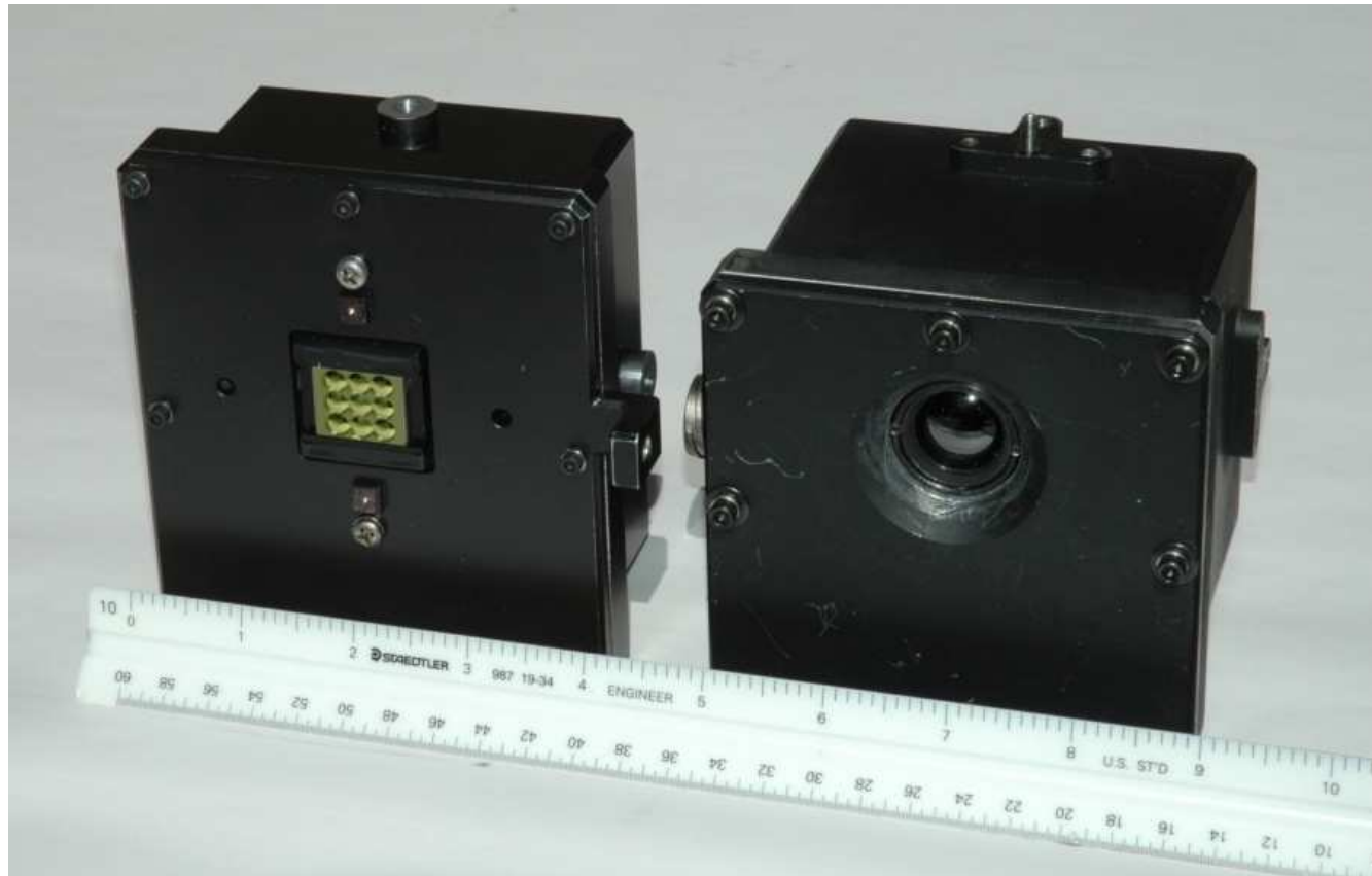
COMP-I Multiple Aperture Camera (left) vs. Single Lens Camera (right)
