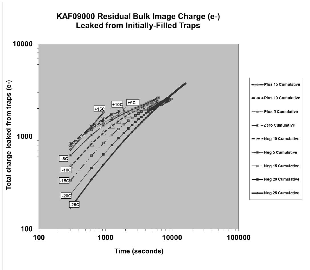
Figure 3: Cumulative Charge Leakage
