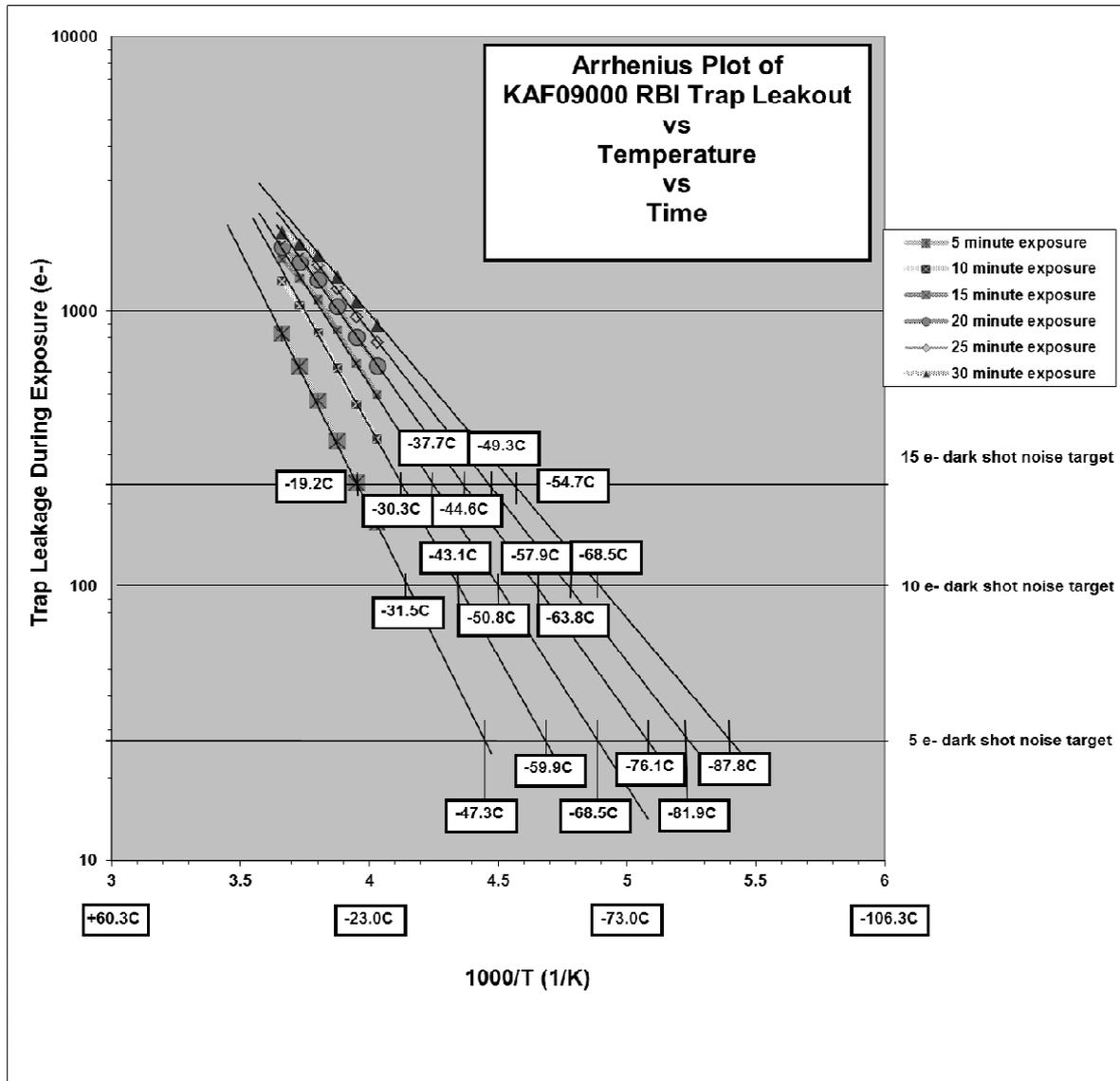
Figure 7: Arrhenius Plot showing trap leakage versus temperature for various exposure times
