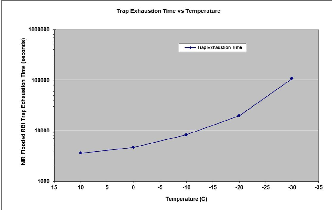
Figure 5: Time to trap exhaustion
