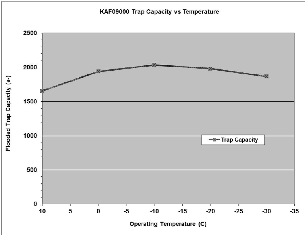
Figure 4: Trap capacity vs operating temperature
