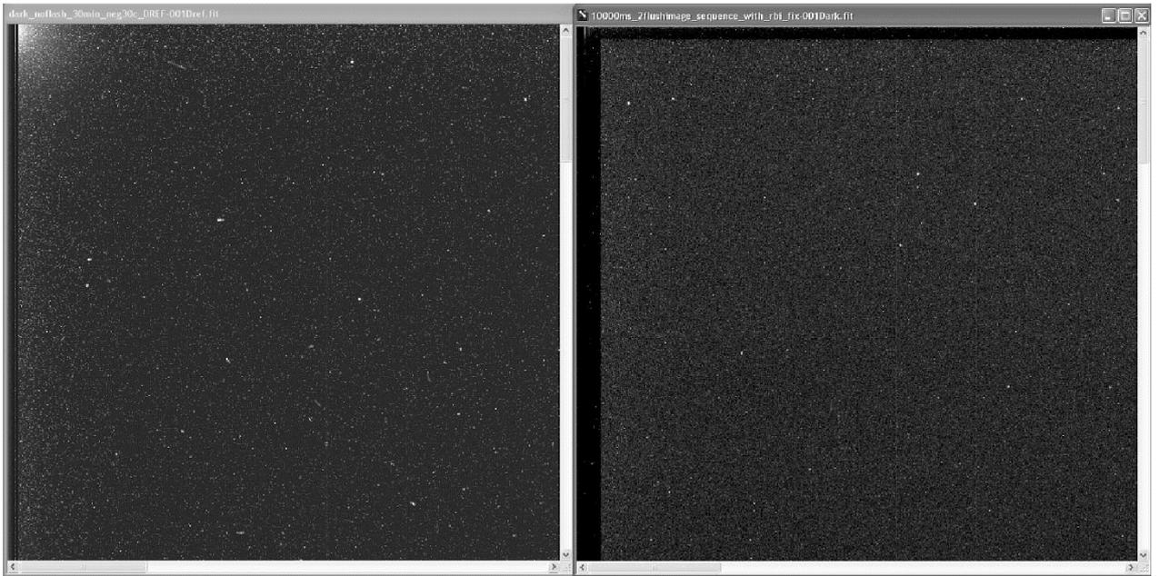
No Light Flood: Shows Amplifier Luminescence      With Light Flood: No Luminescence
