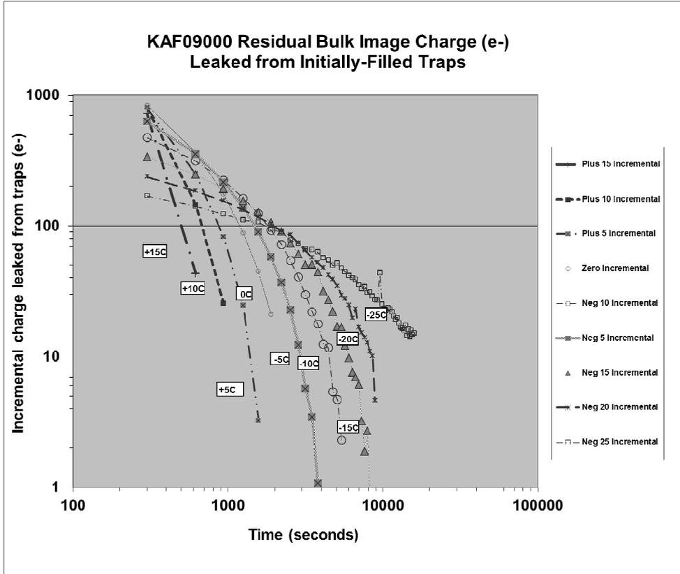
Figure 2: Incremental Charge Leakage (frame to frame)
