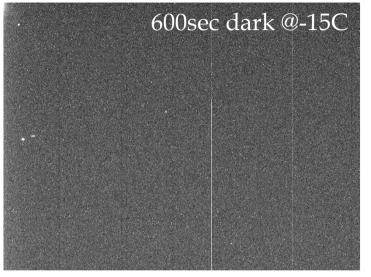
Sensor was grade 1 when deployed Some bad columns developed later
