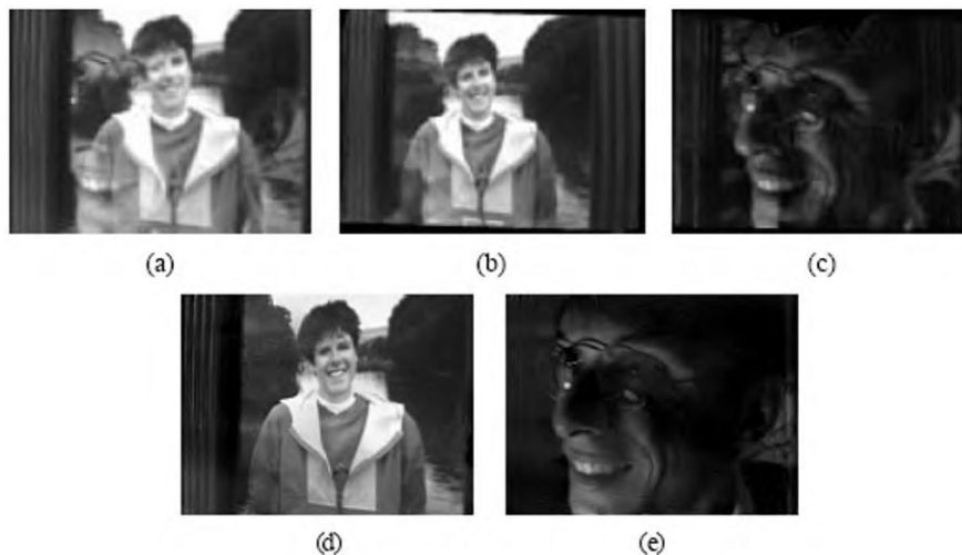
Figure 8.17 Light reflecting off the transparent glass of a picture frame: (a) first image from the input sequence; (b) dominant motion layer min-composite ; (c) secondary motion residual layer max-composite ; (d–e) final estimated picture and reflection layers. The original images are from Black and Anandan (1996), while the separated layers are from Szeliski, Avidan, and Anandan (2000) © 2000 IEEE.
