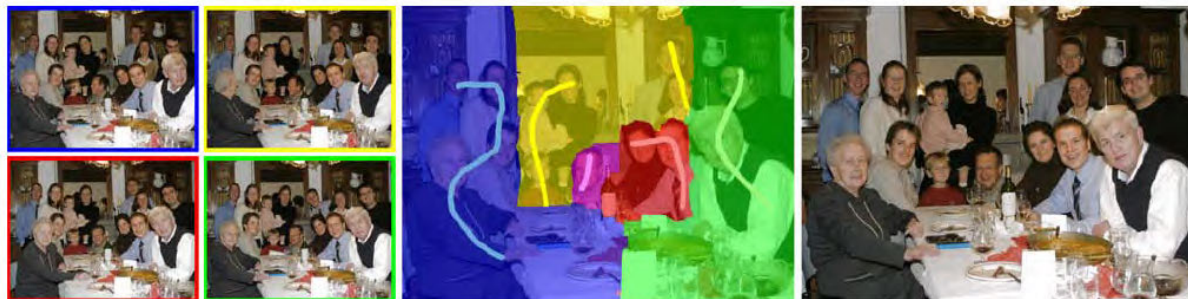
Figure 3.60 An unordered label MRF (Agarwala, Dontcheva, Agrawala et al. 2004) © 2004 ACM: Strokes in each of the source images on the left are used as constraints on an MRF optimization, which is solved using graph cuts. The resulting multi-valued label field is shown as a color overlay in the middle image, and the final composite is shown on the right.
