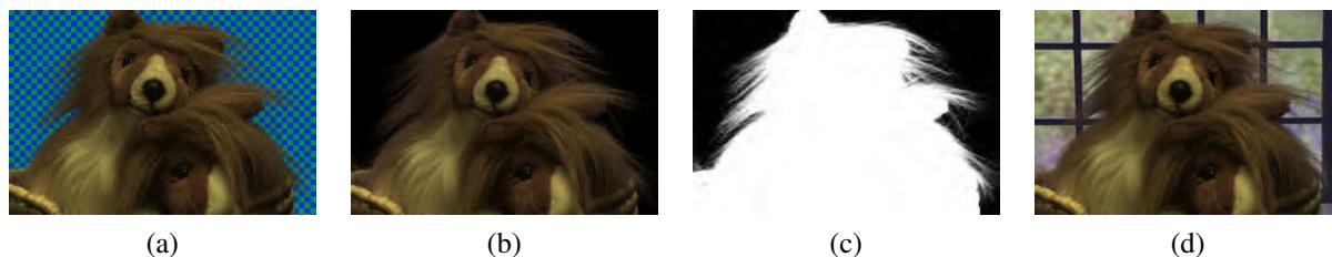
Figure 3.4 Image matting and compositing (Chuang, Curless, Salesin et al. 2001) © 2001 IEEE: (a) source image; (b) extracted foreground object F ; (c) alpha matte \alpha shown in grayscale; (d) new composite C .
