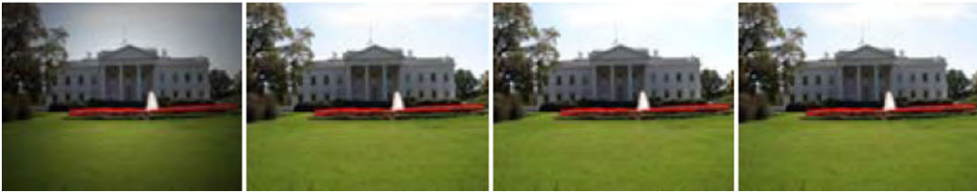
Figure 10.5 Single image vignetting correction (Zheng, Yu, Kang et al. 2008) © 2008 IEEE: (a) original image with strong visible vignetting; (b) vignetting compensation as described by Zheng, Zhou, Georgescu et al. (2006); (c–d) vignetting compensation as described by Zheng, Yu, Kang et al. (2008).
