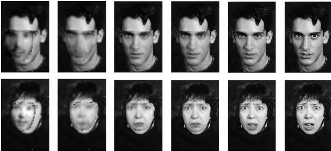
Figure 14.23 Multiresolution model fitting (search) in active appearance models (Cootes, Edwards, and Taylor 2001) © 2001 IEEE. The columns show the initial model, the results after 3, 8, and 11 iterations, and the final convergence. The rightmost column shows the input image.
