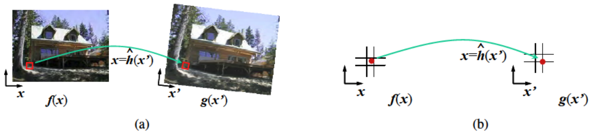
Figure 3.47 Inverse warping algorithm: (a) a pixel g(x') is sampled from its corresponding location x = \hat{h}(x') in image f(x) ; (b) detail of the source and destination pixel locations.
