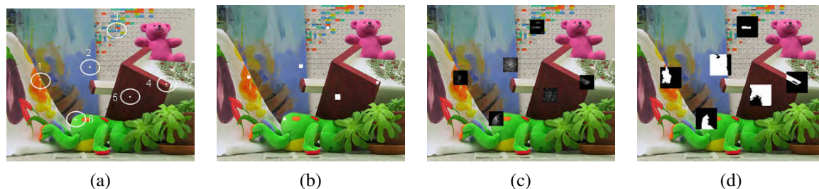
Figure 11.9 Aggregation window sizes and weights adapted to image content (Tombari, Mattocchia, Di Stefano et al. 2008) © 2008 IEEE: (a) original image with selected evaluation points; (b) variable windows (Veksler 2003); (c) adaptive weights (Yoon and Kweon 2006); (d) segmentation-based (Tombari, Mattocchia, and Di Stefano 2007). Notice how the adaptive weights and segmentation-based techniques adapt their support to similarly colored pixels.
