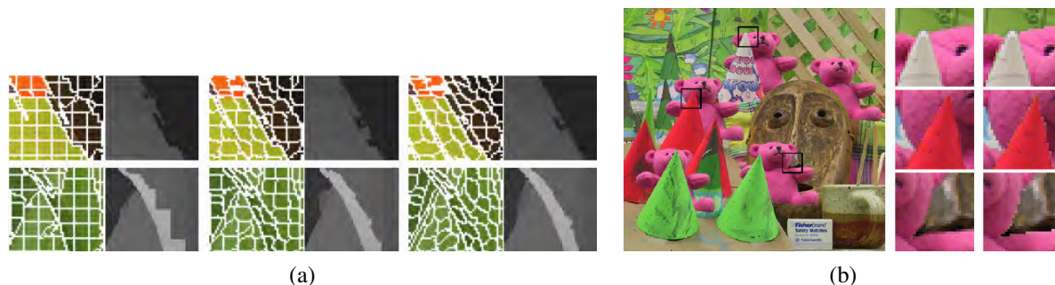
Figure 11.13 Stereo matching with adaptive over-segmentation and matting (Taguchi, Wilburn, and Zitnick 2008) © 2008 IEEE: (a) segment boundaries are refined during the optimization, leading to more accurate results (e.g., the thin green leaf in the bottom row); (b) alpha mattes are extracted at segment boundaries, which leads to visually better compositing results (middle column).
