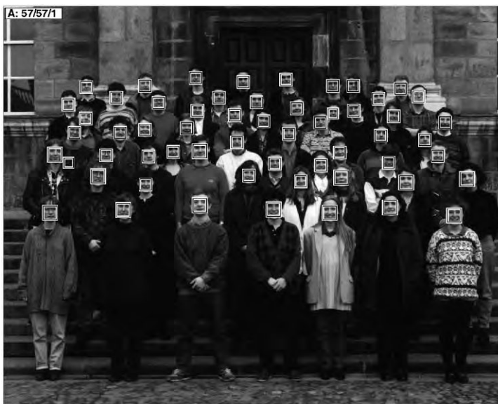
Figure 14.2 Face detection results produced by Rowley, Baluja, and Kanade (1998a) © 1998 IEEE. Can you find the one false positive (a box around a non-face) among the 57 true positive results?
