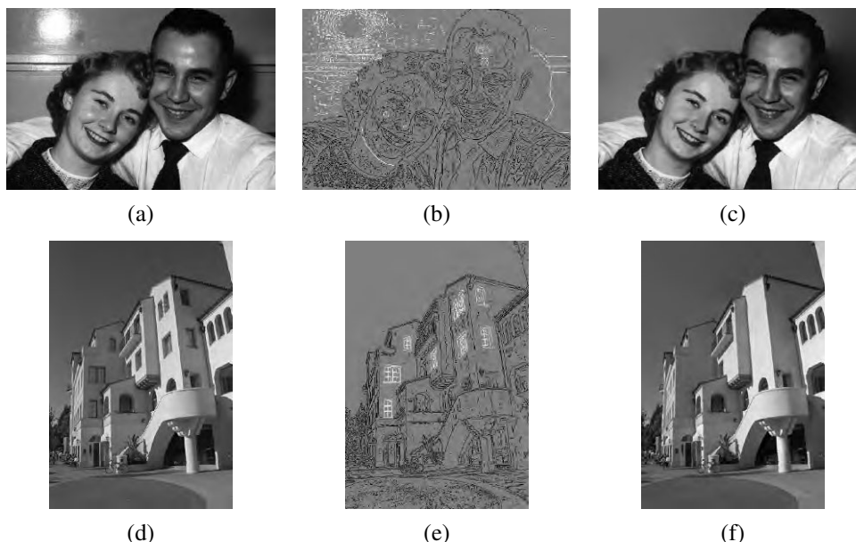
Figure 4.39 Image editing in the contour domain (Elder and Goldberg 2001) © 2001 IEEE: (a) and (d) original images; (b) and (e) extracted edges (edges to be deleted are marked in white); (c) and (f) reconstructed edited images.
