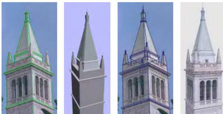
Figure 12.14 Interactive architectural modeling using the Façade system (Debevec, Taylor, and Malik 1996) © 1996 ACM: (a) input image with user-drawn edges shown in green; (b) shaded 3D solid model; (c) geometric primitives overlaid onto the input image; (d) final view-dependent, texture-mapped 3D model.
