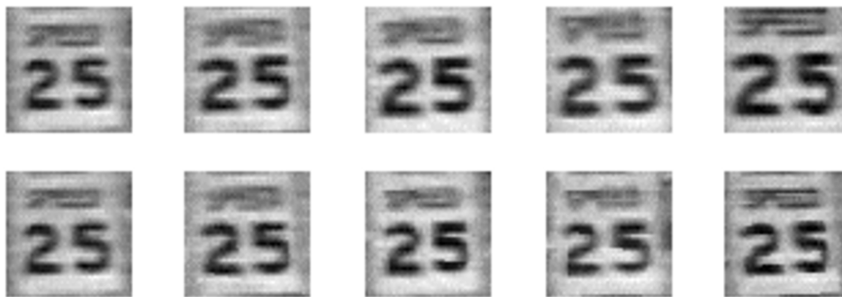
Figure 4.28 Feature tracking using an affine motion model (Shi and Tomasi 1994) © 1994 IEEE, Top row: image patch around the tracked feature location. Bottom row: image patch after warping back toward the first frame using an affine deformation. Even though the speed sign gets larger from frame to frame, the affine transformation maintains a good resemblance between the original and subsequent tracked frames.
