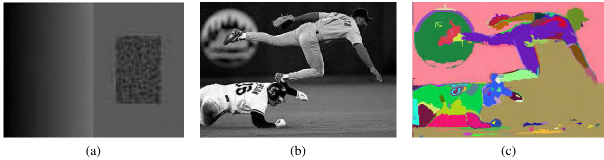
Figure 5.14 Graph-based merging segmentation (Felzenszwalb and Huttenlocher 2004b) © 2004 Springer: (a) input grayscale image that is successfully segmented into three regions even though the variation inside the smaller rectangle is larger than the variation across the middle edge; (b) input grayscale image; (c) resulting segmentation using an \mathcal{N}_8 pixel neighborhood.
