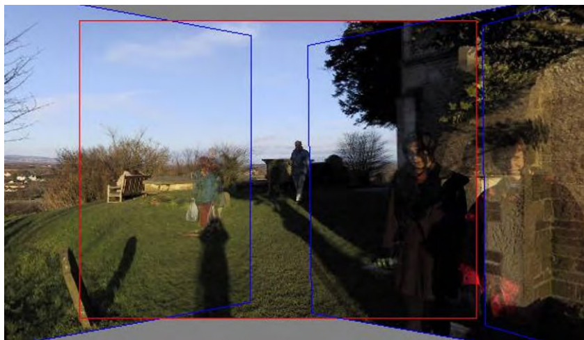
Figure 9.13 Validation of image matches by direct pixel error comparison can fail when the scene contains moving objects (Uyttendaele, Eden, and Szeliski 2001) © 2001 IEEE.
