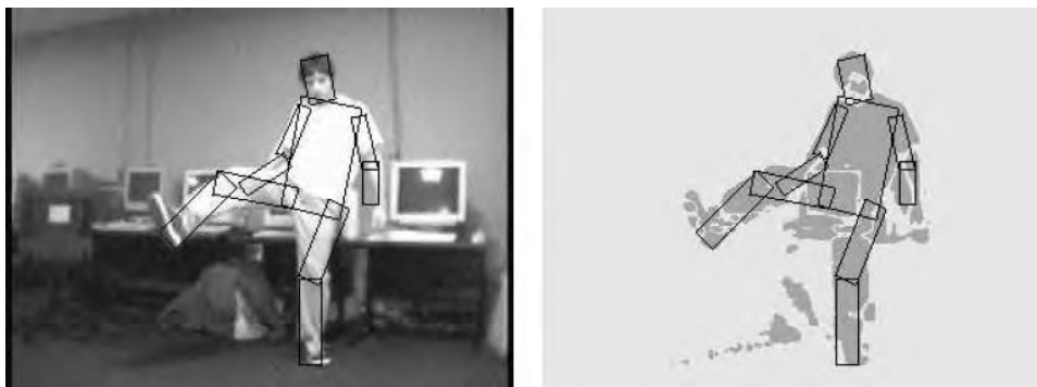
Figure 14.40 Using pictorial structures to locate and track a person (Felzenszwalb and Huttenlocher 2005) © 2005 Springer. The structure consists of articulated rectangular body parts (torso, head, and limbs) connected in a tree topology that encodes relative part positions and orientations. To fit a pictorial structure model, a binary silhouette image is first computed using background subtraction.
