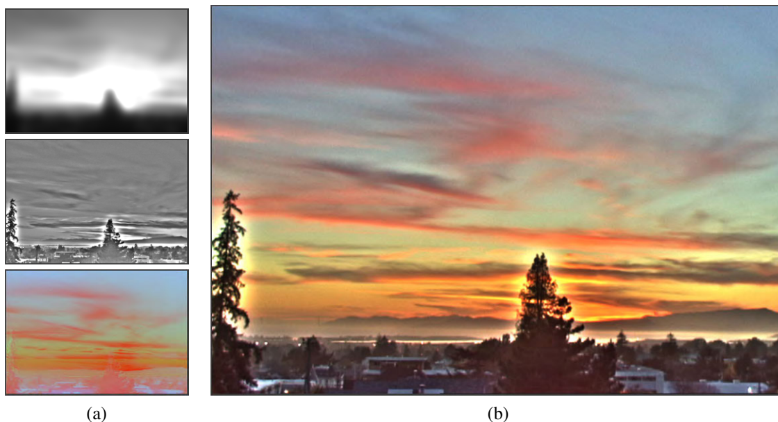
Figure 10.21 Local tone mapping using linear filters: (a) low-pass and high-pass filtered log luminance images and color (chrominance) image; (b) resulting tone-mapped image (after attenuating the low-pass log luminance image) shows visible halos around the trees. Processed images courtesy of Frédo Durand, MIT 6.815/6.865 course on Computational Photography.
