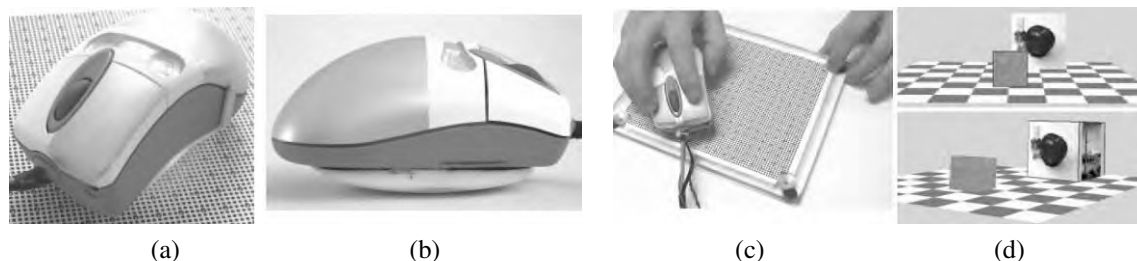
Figure 6.6 The VideoMouse can sense six degrees of freedom relative to a specially printed mouse pad using its embedded camera (Hinckley, Sinclair, Hanson et al. 1999) © 1999 ACM: (a) top view of the mouse; (b) view of the mouse showing the curved base for rocking; (c) moving the mouse pad with the other hand extends the interaction capabilities; (d) the resulting movement seen on the screen.
