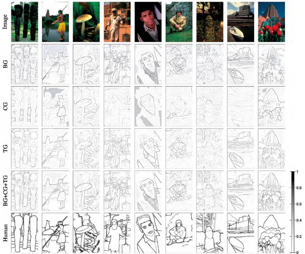
Figure 4.33 Combined brightness, color, texture boundary detector (Martin, Fowlkes, and Malik 2004) © 2004 IEEE. Successive rows show the outputs of the brightness gradient (BG), color gradient (CG), texture gradient (TG), and combined (BG+CG+TG) detectors. The final row shows human-labeled boundaries derived from a database of hand-segmented images (Martin, Fowlkes, Tal et al. 2001).
