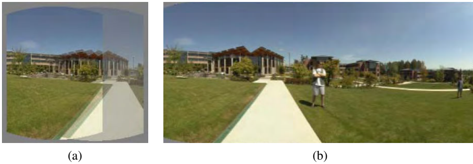
Figure 9.8 A cylindrical panorama (Szeliski and Shum 1997) © 1997 ACM: (a) two cylindrically warped images related by a horizontal translation; (b) part of a cylindrical panorama composited from a sequence of images.
