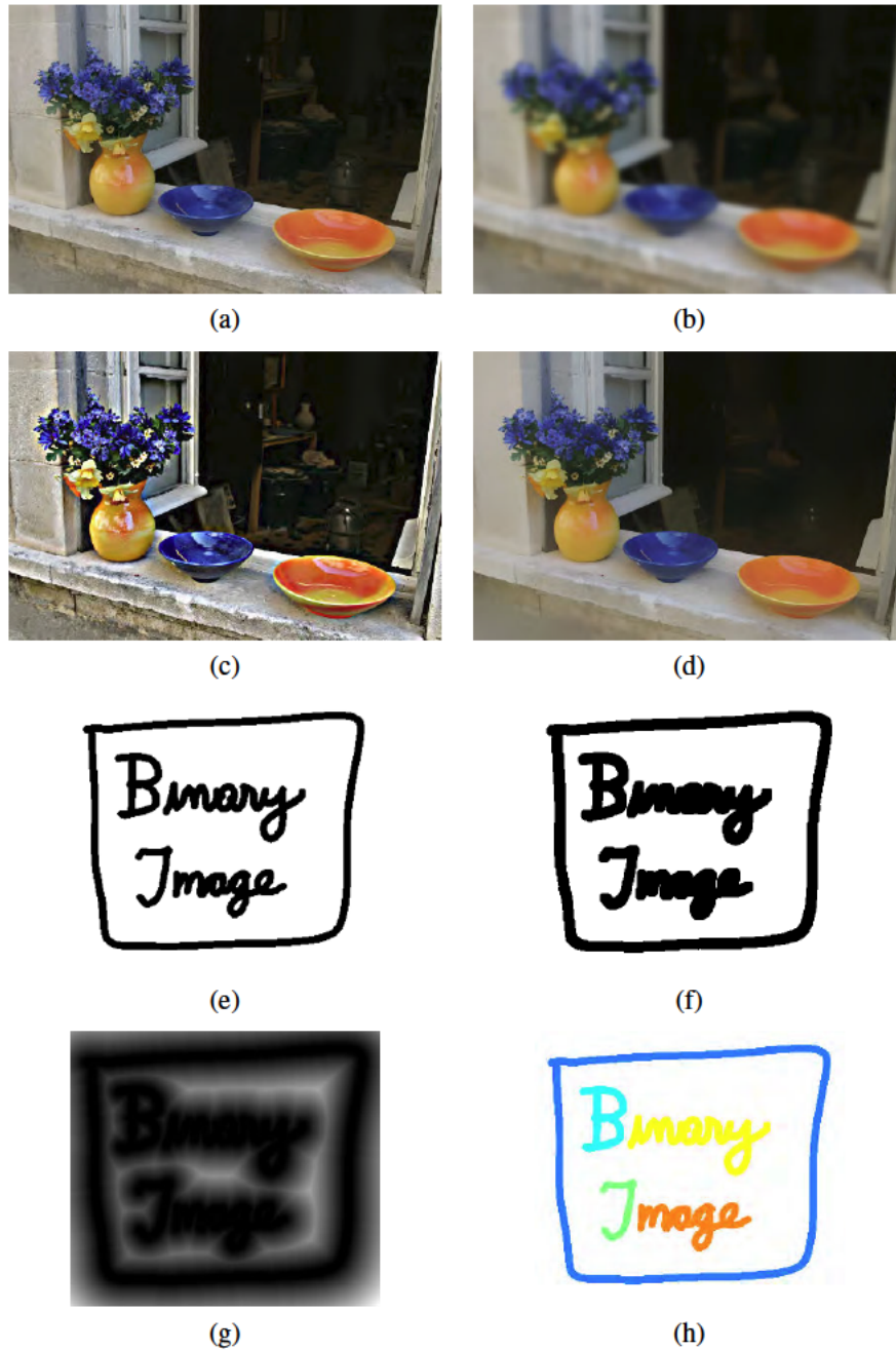
Figure 3.11 Some neighborhood operations: (a) original image; (b) blurred; (c) sharpened; (d) smoothed with edge-preserving filter; (e) binary image; (f) dilated; (g) distance transform; (h) connected components. For the dilation and connected components, black (ink) pixels are assumed to be active, i.e., to have a value of 1 in Equations (3.41–3.45).
