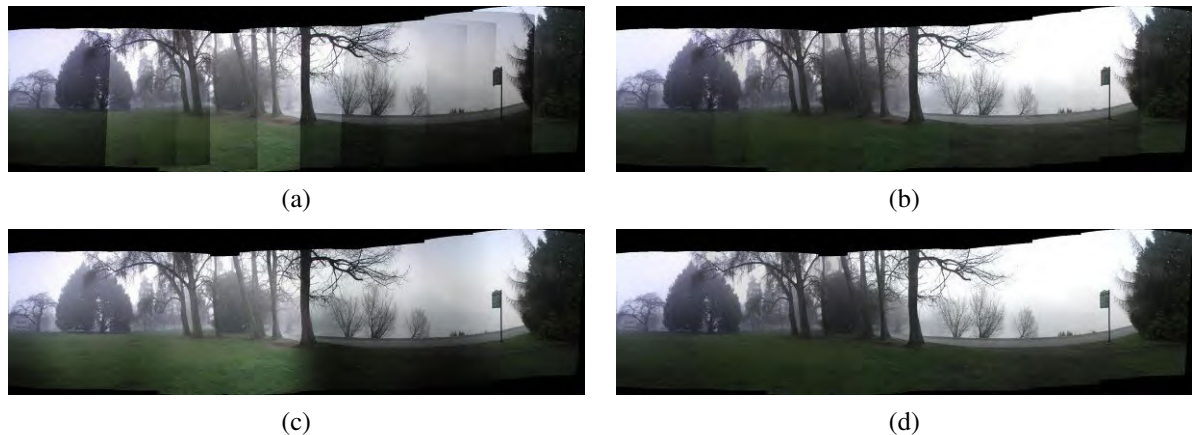
Figure 10.6 Simultaneous estimation of vignetting, exposure, and radiometric response (Goldman 2011) © 2011 IEEE: (a) original average of the input images; (b) after compensating for vignetting; (c) using gradient domain blending only (note the remaining mottled look); (d) after both vignetting compensation and blending.
