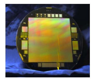
vertical binning. For both frame transfer configurations, the charge may be read out through the eight amplifiers at the bottom or top of the image frame storage region
