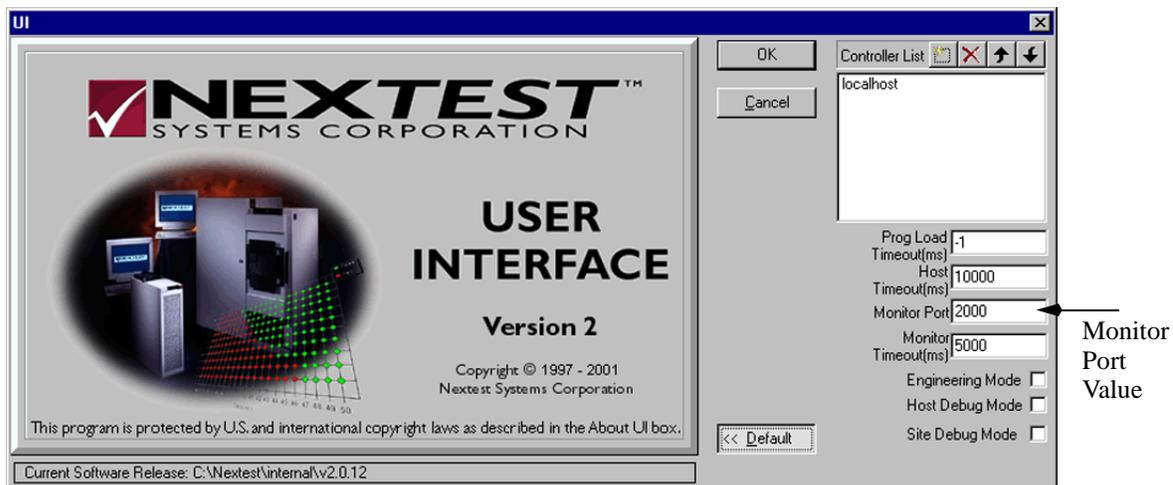
`ui_MonitorPort` can be used from a Windows command line, or from within a batch file (see [ui\\_BatchFile](#)). While it is possible to use `ui_MonitorPort` from user-written C-code this has limited value. Setting a new value from C-code has no effect until the next test program is loaded.
