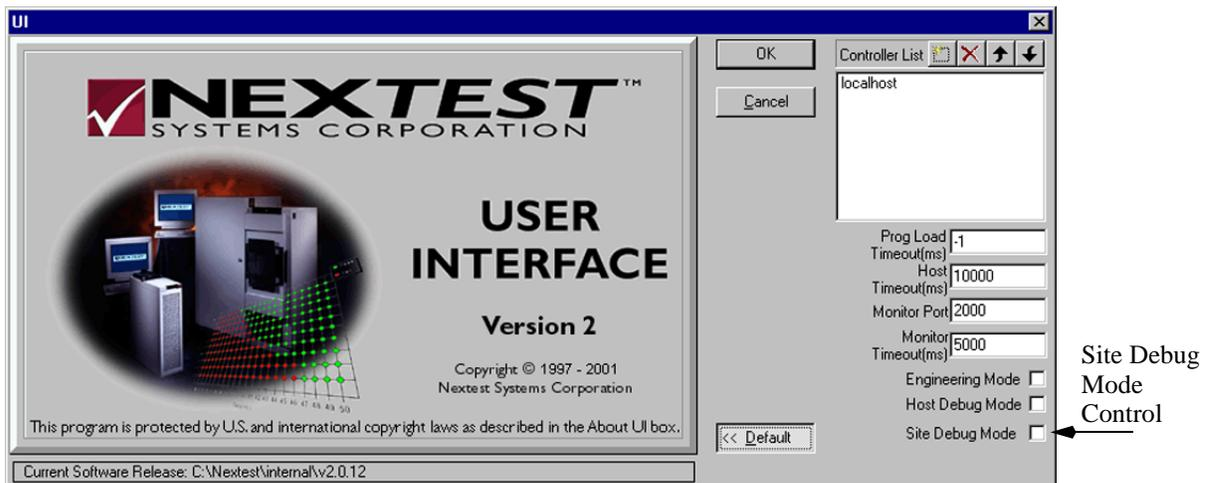
This mode is normally set using the UI graphic interface (above) but can also be done using `ui_SiteDebug`.
