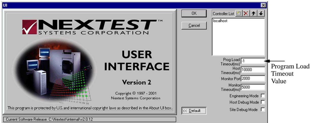
`ui_LoadTimeOut` can be used from a Windows command line, or from within a batch file (see [ui\\_BatchFile](#)). While it is possible to use `ui_LoadTimeOut` from user-written C-code this has limited value. Setting a new value from C-code has no effect until the next test program is loaded.
