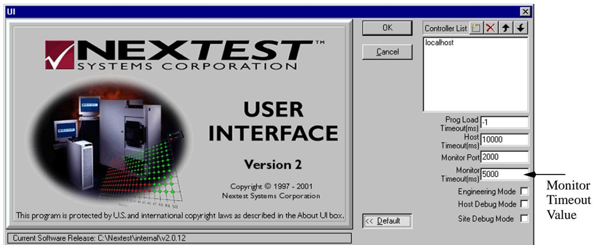
`ui_MonitorTimeOut` can be used from a Windows command line, or from within a batch file (see [ui\\_BatchFile](#)). While it is possible to use `ui_MonitorTimeOut` from user-written C-code this has limited value. Setting a new value from C-code has no effect until the next test program is loaded.
