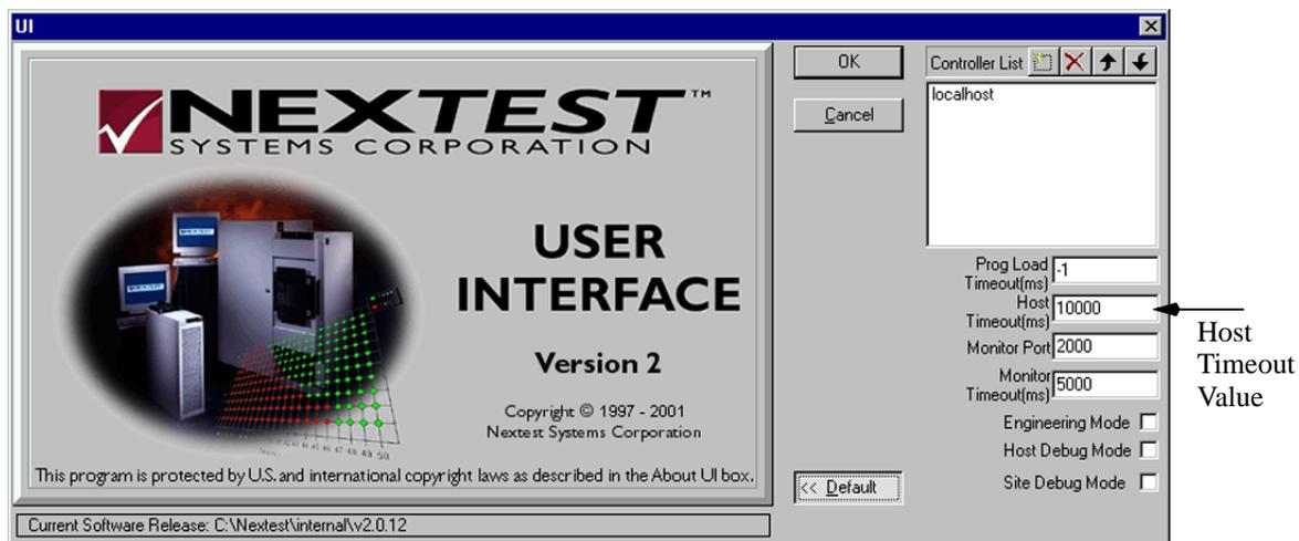
`ui_HostTimeOut` can be used from a Windows command line, or from within a batch file (see [ui\\_BatchFile](#)). While it is possible to use `ui_HostTimeOut` from user-written C-code this has limited value. Setting a new value from C-code has no effect until the next test program is loaded.
