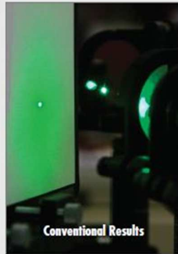
Figure 1: Light reflected by an object outside FOV being scattered from the edges of a lens without edge blackening
