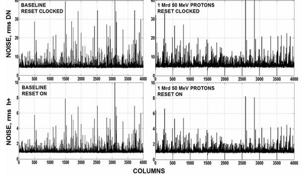
Fig. 28. Read noise before and after proton irradiation.
