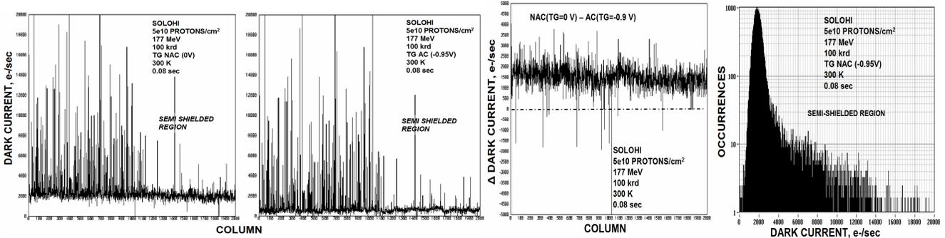
Fig. 39a/b. 177 MeV proton damaged responses.
