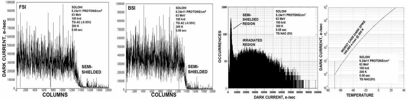
Fig. 37a/b. Dark video traces for FSI and BSI SoloHi imager.
