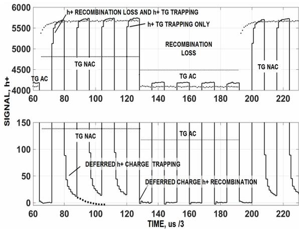
Fig. 49. TG recombination loss and deferred charge.
