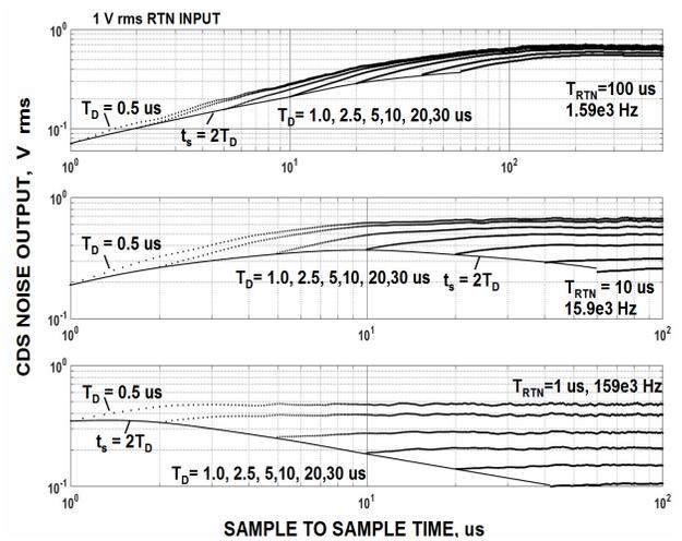
Fig. 12. CDS RTN noise response as a function of  $t_s$ ,  $T_D$  and  $\tau_{RTN}$ .
