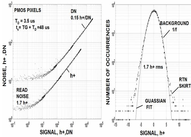
Fig. 15 a/b. PTC and read noise histogram.
