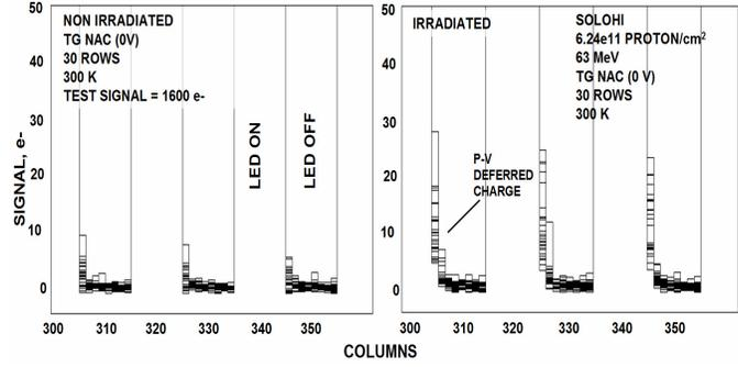
Fig. 41a,b. Raw and CDS lack of offset shift after irradiation. Fig. 42a,b. Deferred charge increase due to proton induced P-V traps.
