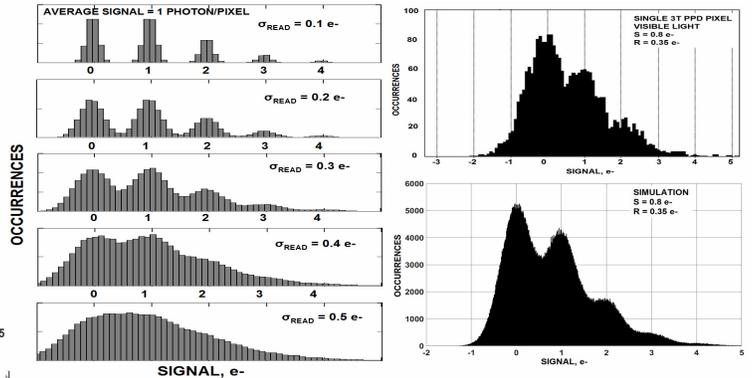
Fig. 30. Single photon counting quantized histograms.
