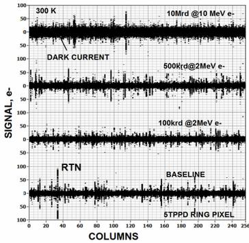
Fig. 27. Read noise at different irradiated dose levels.
