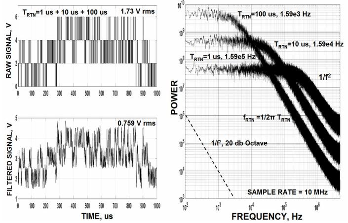
Fig. 10a/b. RTN time and frequency responses for three different  $\tau_{RTN}$ .
