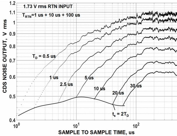
Fig. 13. CDS noise as function  $t_s$  and  $\tau_D$  for three  $\tau_{RTN}$ .
