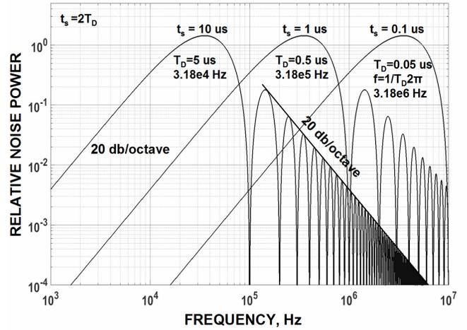
**Fig. 2.** CDS transfer function for three  $t_s$ .
