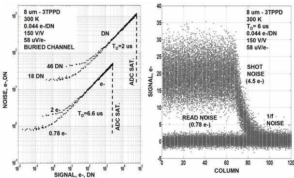
Fig. 31a/b. PTC Sub electron noise PT curve.
