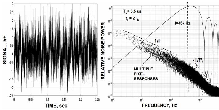
Fig. 25a/b. Pixel flicker noise and spectral noise for different pixels.
