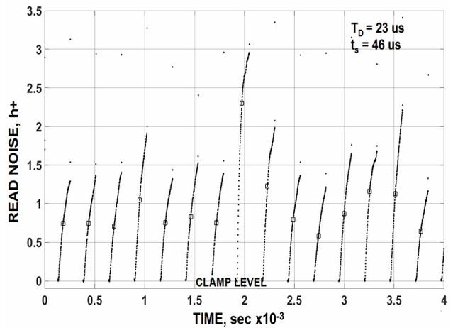
Fig. 20. Clamped video showing noise increase with time for  $\tau_D$
