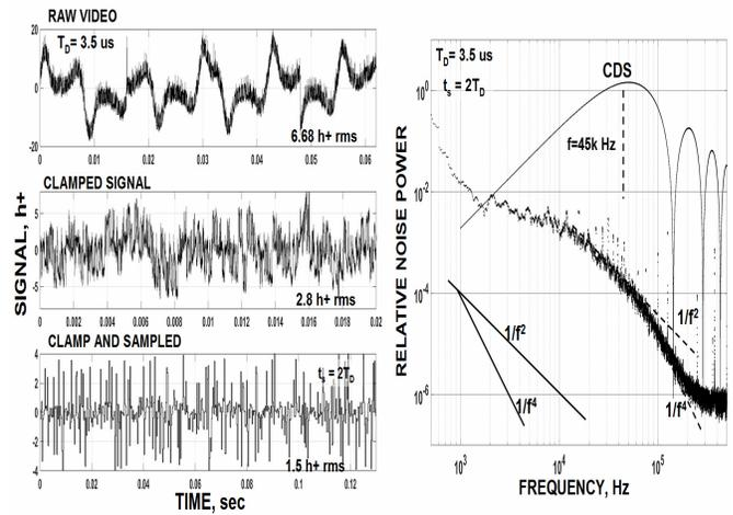
Fig. 22a/b. Raw, clamped, and sampled video and spectral response.
