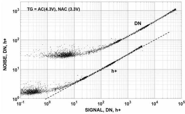
Fig. 51a,b. PT curve for an imager without TG loss. charge.
