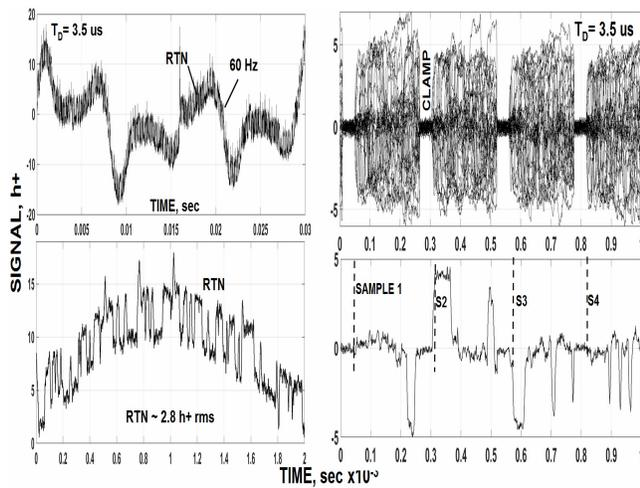
Fig. 21a/b. Raw 60 Hz and RTN and clamped video response.
