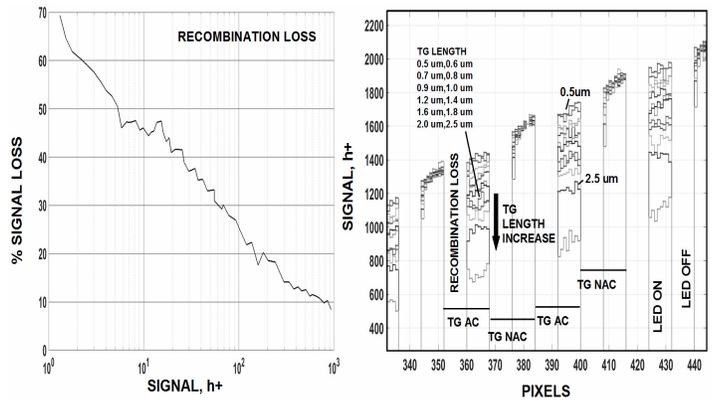
Fig. 50a,b. TG recombination loss versus signal and TG gate width.
