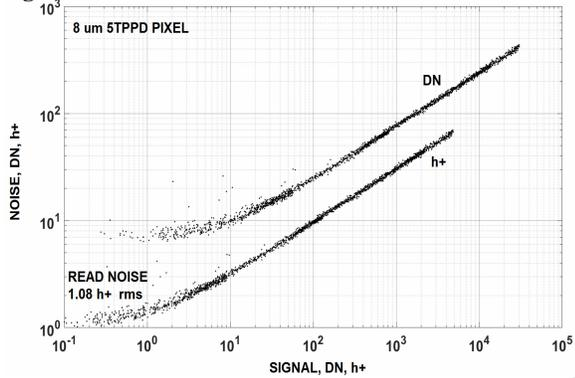
Fig. 29. PT curve demonstrating 1 h+ rms read noise.
