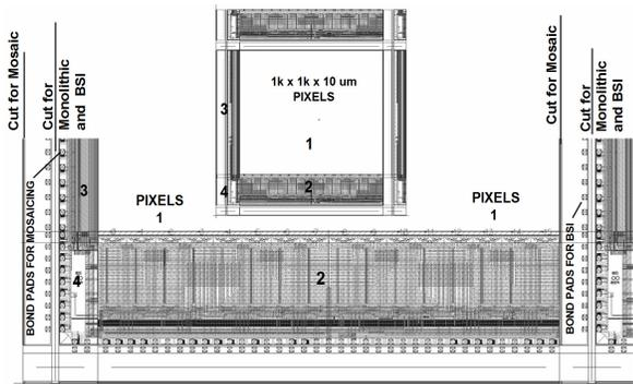
Fig. 45. Mk x Nk dicing for monolithic and mosaicing.
