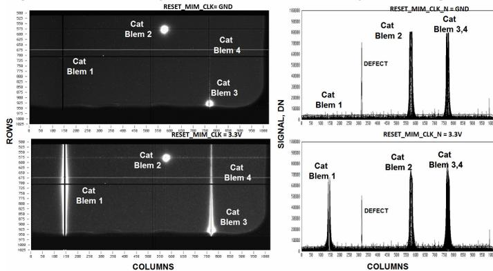
Fig. 47a,b. An erupting Cat Blem caused by change in pixel voltage.
