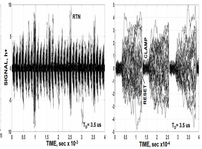
Fig. 16a/b. Clamped video for several pixels.
