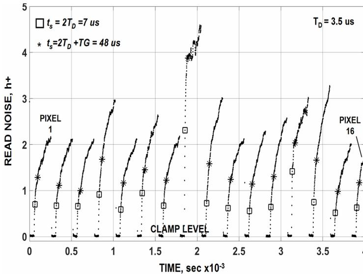
Fig. 17. Clamped video showing noise increase with time.
