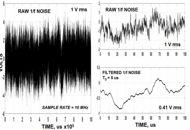
**Fig. 4a,b.** Raw 1/f noise and filtered 1/f noise.
