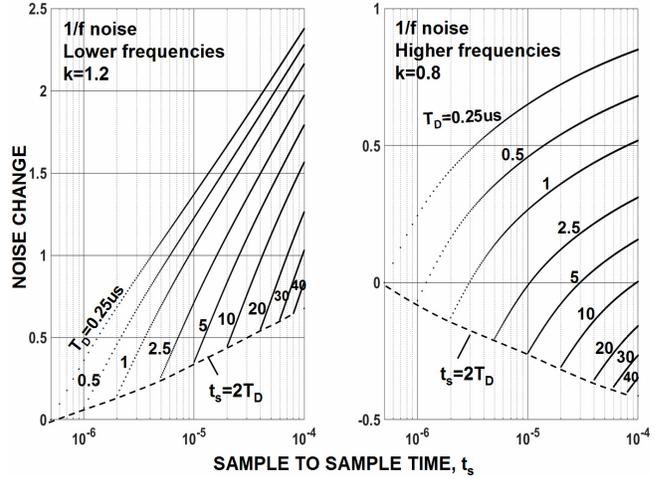
Fig. 8a/b. CDS noise change for different sloped 1/f noise.
