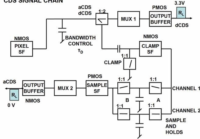
**Fig. 1.** Pixel CDS signal processor.
