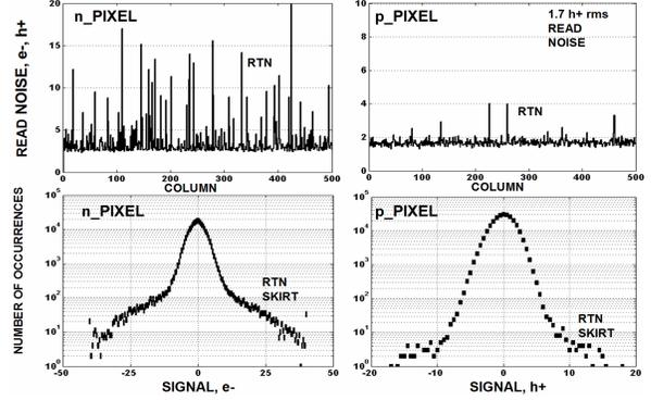
Fig. 26a/b. NMOS and PMOS RTN comparison.
