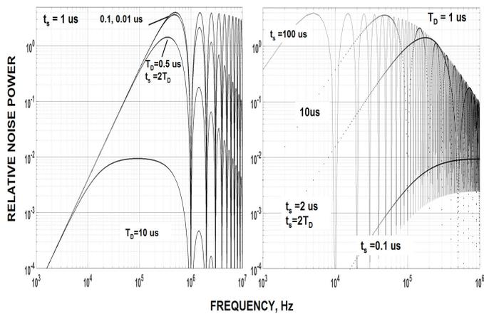
**Fig. 3a,b.** CDS transfer functions for different  $\tau_D$  and  $t_s$ .
