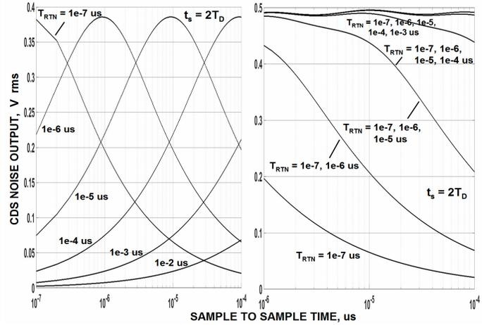
Fig. 14a/b. CDS noise as function  $t_s$  and  $\tau_D$  for many different  $\tau_{RTN}$ .
