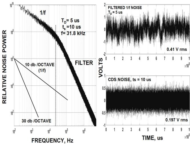
**Fig. 5a,b.** Filtered 1/f frequency response and CDS output noise.
