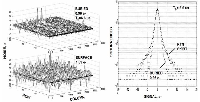
Fig. 32a/b. Read noise for surface and buried channel SF MOSFETs.
