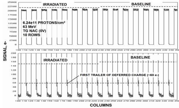
Fig. 43a,b. Deferred charge due to TG traps.
