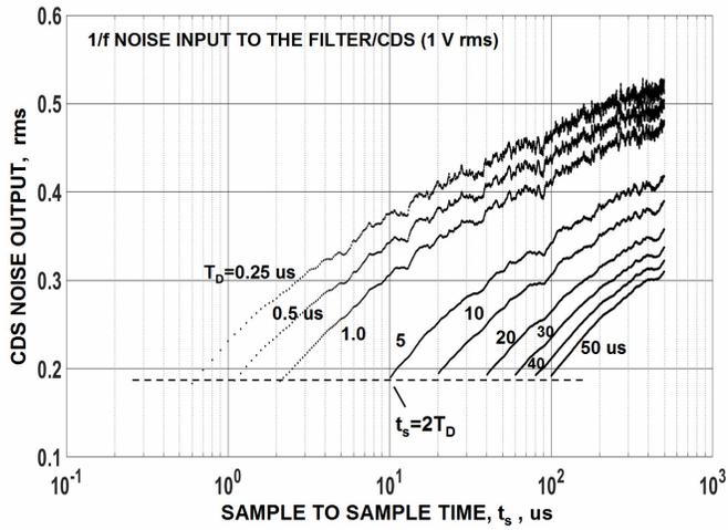
Fig. 7. CDS 1/f noise response as a function of  $t_s$  and  $T_D$ .
