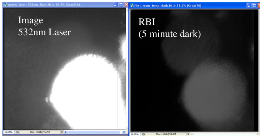
Although weak compared to 656 nm light, at 532 nm there is RBI visible
