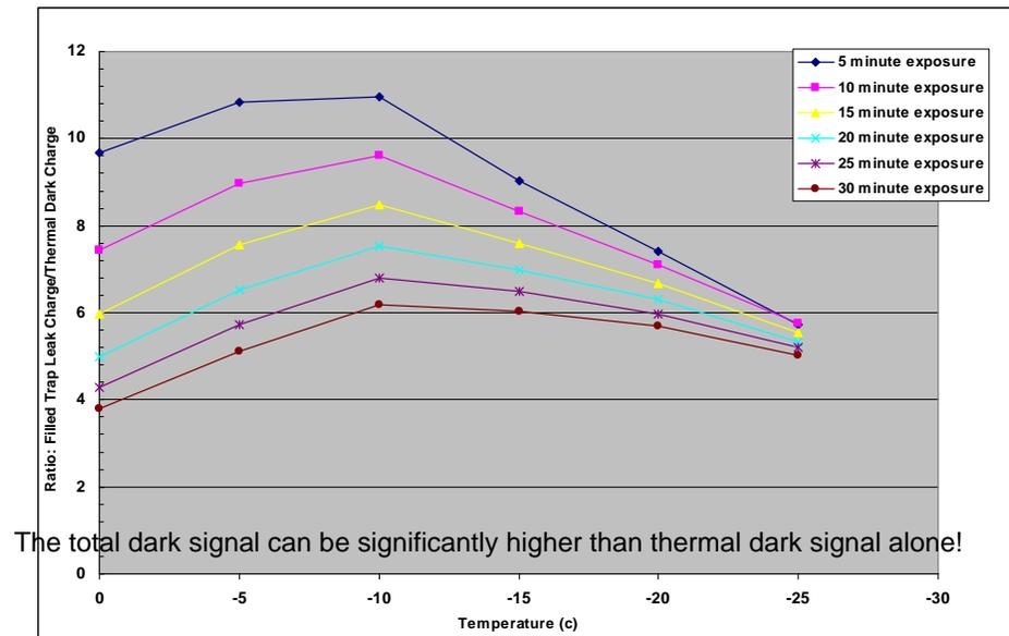
The total dark signal can be significantly higher than thermal dark signal alone!
