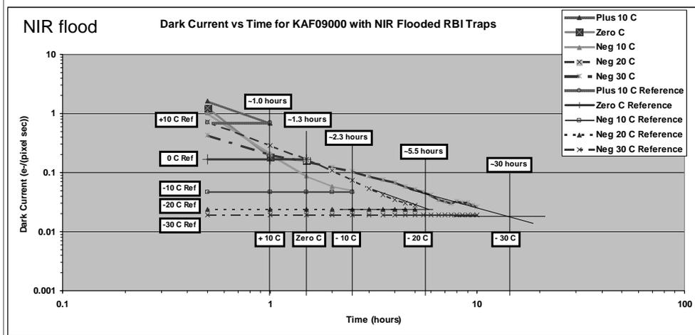
Reference = Current measured in non-flooded case: “cold-start dark” (half hour integrations)
