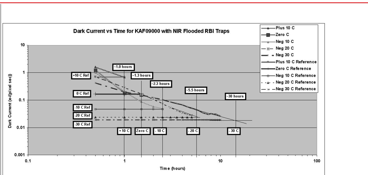
Reference = Current measured in non-flooded case: “cold-start dark”
